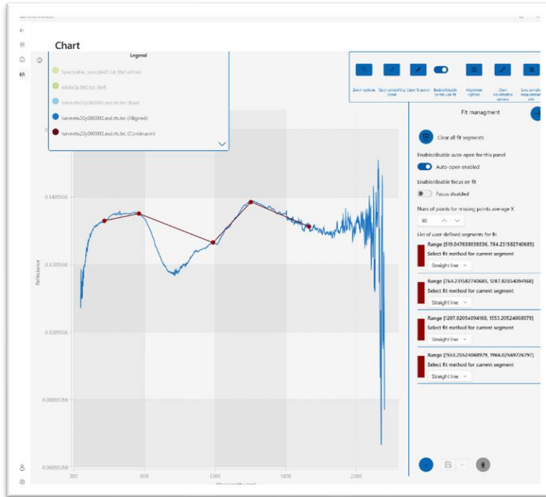
Figure 16 Continuum fitting panel on the right. The list of generated segments is visible in the middle of the panel. At the bottom-left of the panel the button for removing continuum is enabled. In this figure, the legend has been expanded to demonstrate how the list of all loaded or processed spectra is shown.
