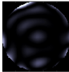
Figure 6: Residual wavefront aberration on the P-WFS arm, after closing the loop with the DM, while keeping the two MALs activated in their best flat shape.
