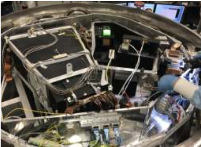
Fig. 4. Actual implementation of the new cross dispersion optics and detectors in the instrument.
