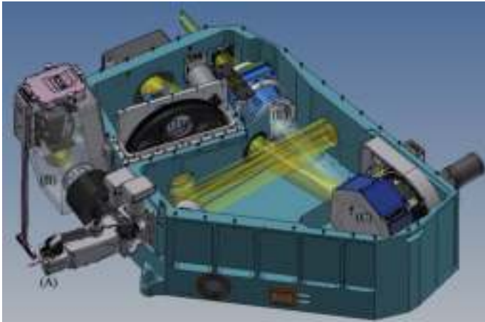
Fig. 3. Top view of the new CRIRES + fore-optics assembly with heat exchangers, jitter mirror unit, SV camera subsystem, slit and decker subsystem, CDU subsystem, camera unit and one of the fixation points.
