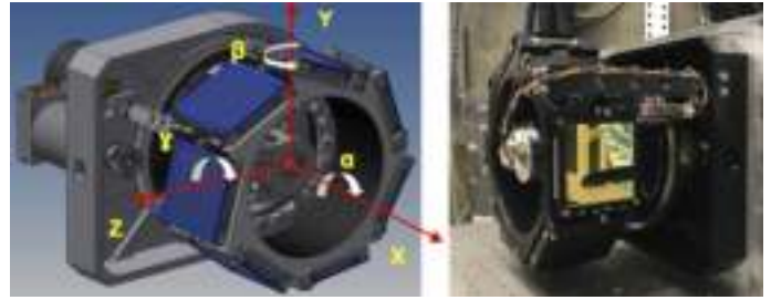
Fig. 5. Grating wheel design with locking mechanism (abandoned and not used in the instrument) and build prototype to verify repeatability and stability.
