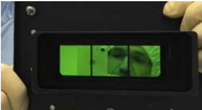
Fig. 10. Three CRIRES+ H2RG detectors arranged as a linear mosaic in the CRIRES+ specific detector mount including the light baffle.
