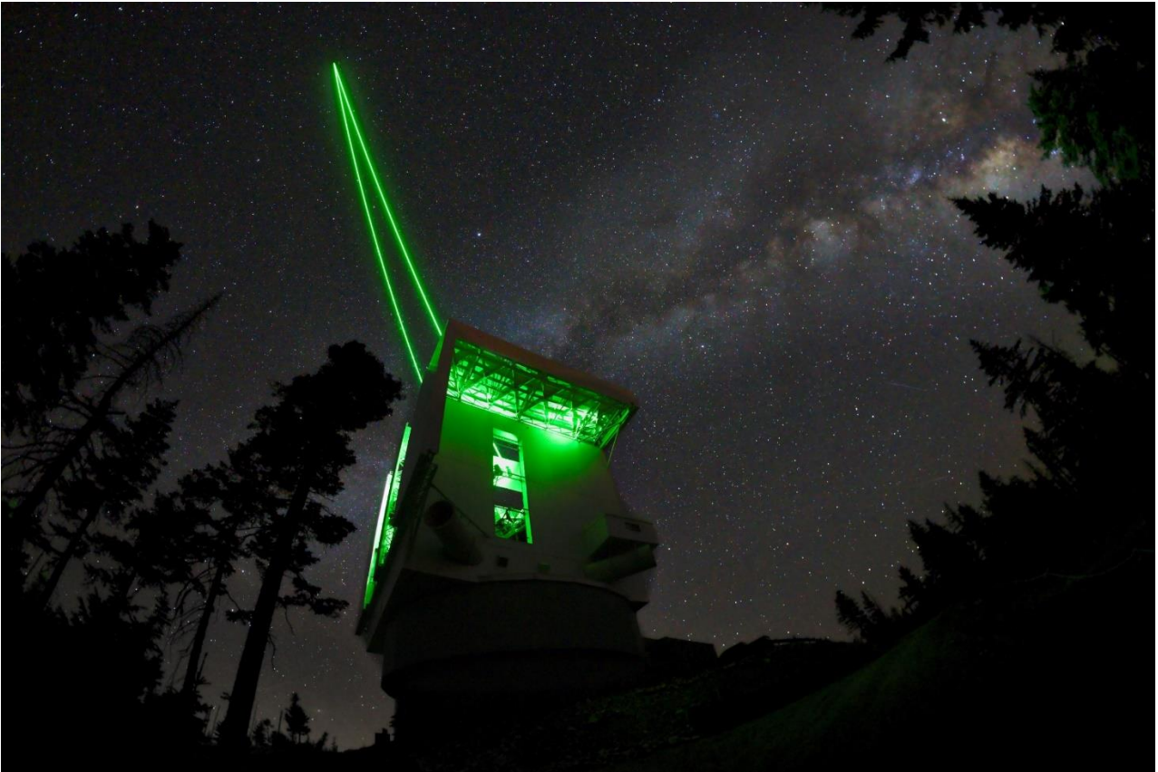
Figure 1: The large binocular telescope with the ARGOS system propagating a bundle of laser beams on each side of the telescope to sky. Each visible beam consists of three individual laser beams forming the constellation of guide stars in the atmosphere. The pulsed Nd:YAG lasers are triggered at 10kHz, with the wavefront sensors adjusted to receive the scattered light from a 12km distance above the telescope.
