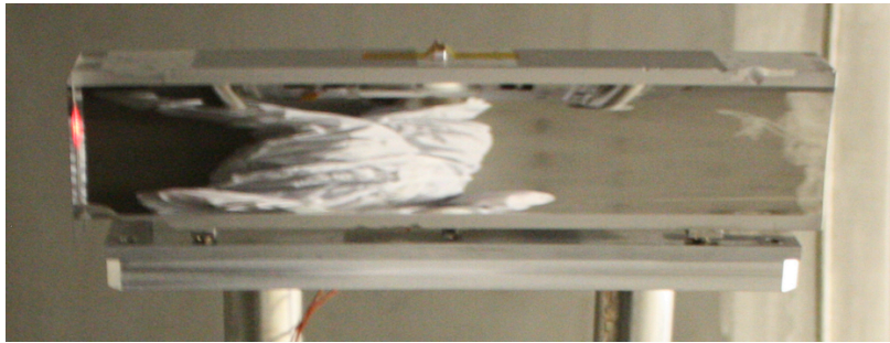
Figure 20: the coated parabola as mounted in the PANTER vacuum chamber (front view).
