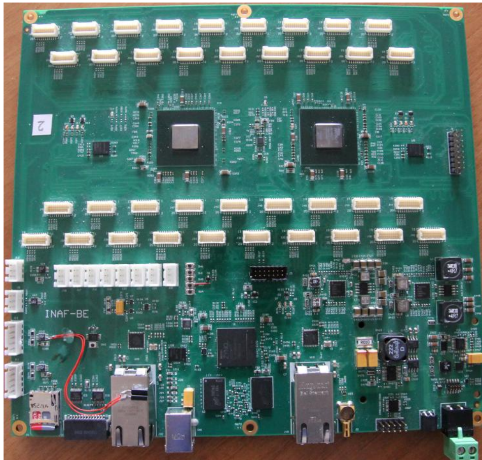
Figure 5 The Back-End Electronics board on-board the ASTRI-Horn camera.
