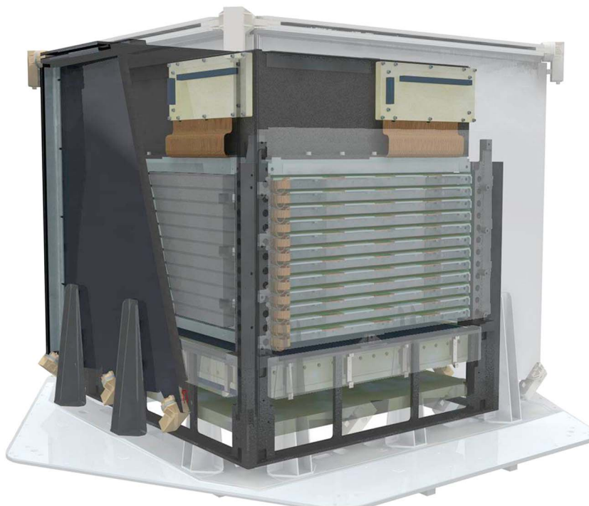
Figure 1. Schematic view of the AGILE instrument [from Tavani et al., 2009 ]. The core of the instrument is provided by the silicon tracker for gamma ray and particle detection in the 10 MeV–10 GeV energy range. On top of it, a very light hard X-ray detector (Super-Agile) is positioned. At the bottom of the Tracker, a Minicalorimeter of CsI(Tl) bars provides additional energy information on the Tracker events and an independent detection device for photons in the range 1–100 MeV. A segmented anticoincidence system made of 12 lateral panels and one top panel of plastic scintillators surrounds the whole detector.
