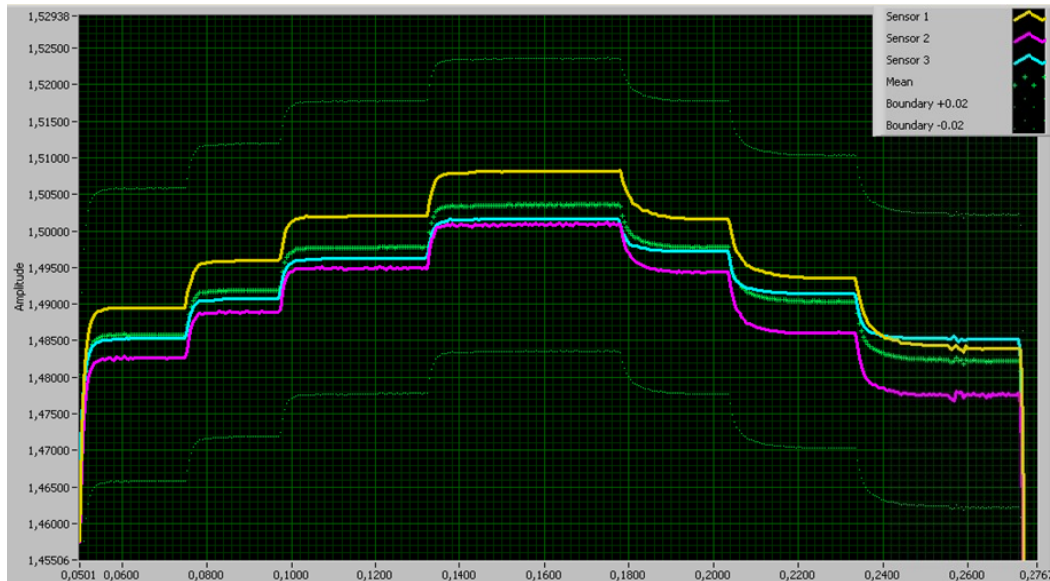
Figure 14: Accuracy without calibration and resolution. Setting at 1.485mm. Steps of 5 \mu m.
