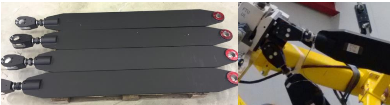
Figure 7: Vanes with tensioners and forks and detail of their attachment to the Stiff finger
