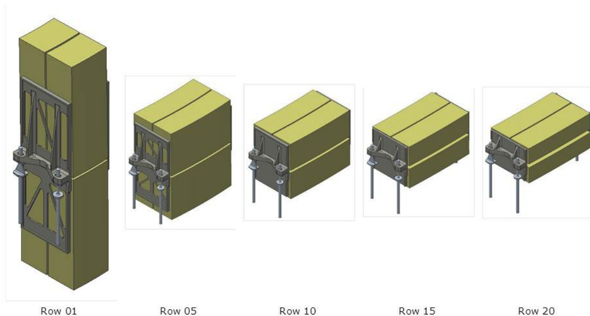
Figure 6: Five examples of MM designs for radii ranging from 0.25 m (row 01) to 1.5 m (row 20).
