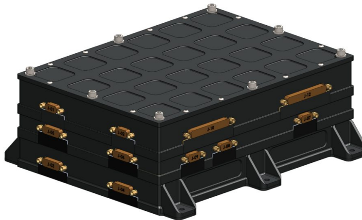
Figure 10: Typical cooler drive electronics box for a two stages compressor set.
