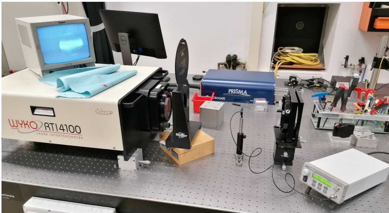
Figure 19: Optical setup used for the optical quality characterization of a LCVR produced by Thorlabs: WYKO RTI 4100 laser interferometer, the LCVR with its benchtop controller and a reference flat mirror.
