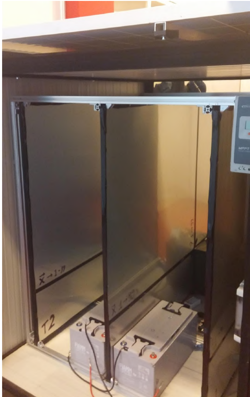
Figure 1: Assembly phase of the telescope. It is possible to see the three sensitive planes fixed vertically on an aluminium frame to keep the alignment inside the external box.
