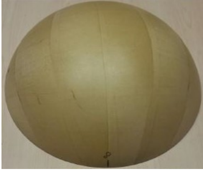
Figure 4. 1mm thick vacuum window developed by NRC (image credited by NRC).
