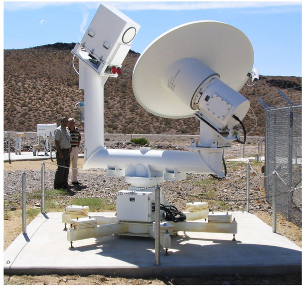
Fig. 4 Advanced Media Calibration unit, installed near DSS 25. The unit delivers, after processing, the path delay due to the water vapor along the line of sight. Hardware with similar functionalities is installed also at ESA's DSA-3
