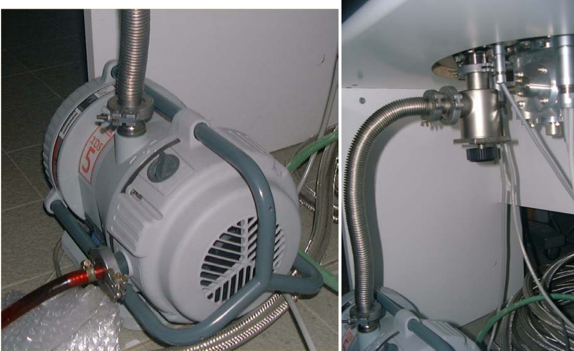
Fig. 3 Vacuum dry pump Boc Edwards XDS5 (left) and connection to the facility by its valve (right)
