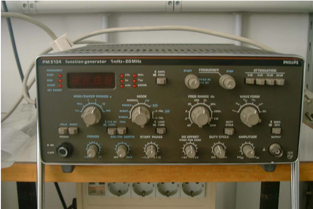
Fig. 4 Philips PM5134 function generator front view
