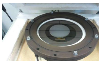
Fig. 8. The setup for the slumping of Eagle glasses on Si 3 N 4 sample mould: the glass was cut to circular shape with diameter suitable for the application of pressure.
