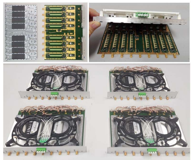
Fig. 6. Photos of the WS RF/IF module. Top left: mechanical housing (left) and fabricated PCB (right) before assembly. Microwave absorbers are glued in the pockets of the PCB mechanical housing. Top right: PCB board (first prototype version) and mechanical housing during assembly with optical transmitters. Bottom: Four WS RF/IF modules fully assembled, with OTXs.
