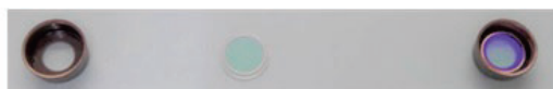
Figure 11. SPS bandpass filter (center) glued on the front window of the SiPM cap (right).
