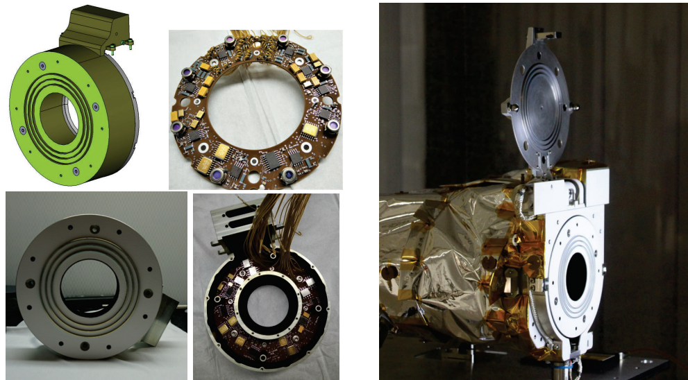
Figure 2. The SPS unit. Left clockwise) 3D CAD rendering of the SPS mechanical flange; the SPS electronics board with the 8 SiPM (front view); the board when inserted into the flange (back view), with the cabling of the output connectors; the assembled SPS. Right) the SPS mounted in front of the ASPIICS telescope during on-ground calibrations (surrounded by the Front Door Assembly).
