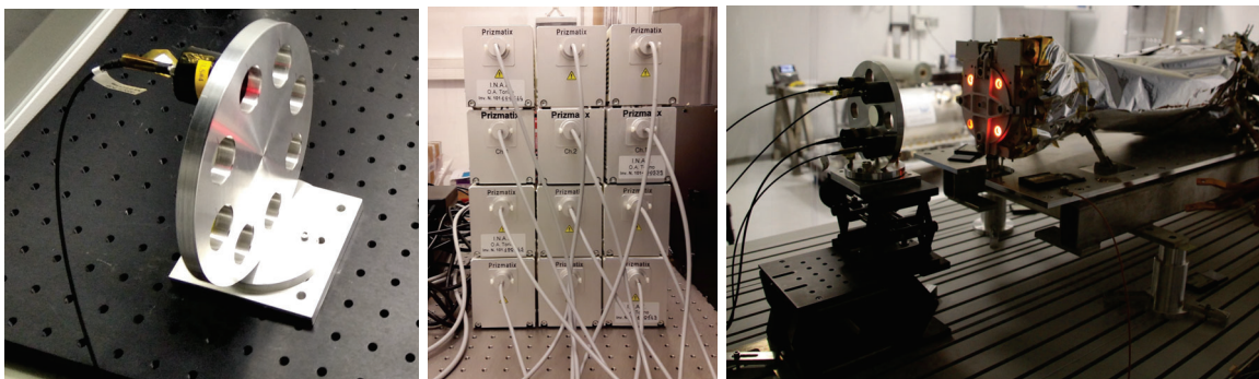
Figure 4. The illumination testbed. Left) The counter-flange adapted to screw the output collimators. Center) The 12 LED units with the optical guides plugged in. Right) Final setup with 4 collimators mounted on the counter-flange and illuminating the SPS channel B, during the SPS calibration campaign.
