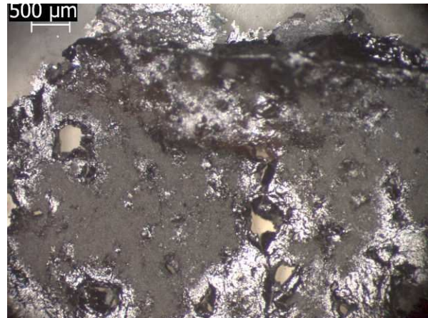
FIGURE 2. Tin plating on chromium: Cr was dissolved and the deposit is inconsistent.
