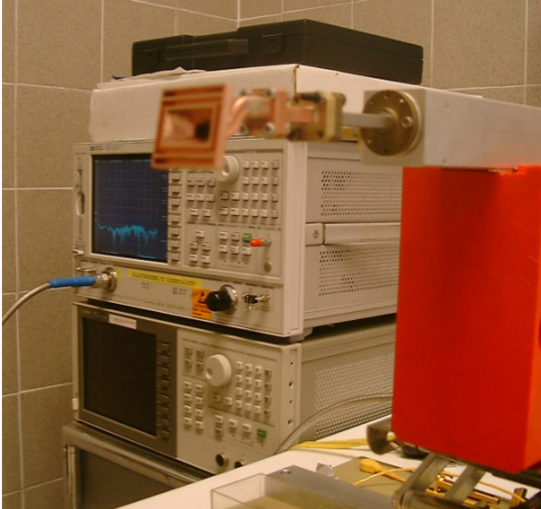
Figure 26 Free space Return Loss measurement for the horns under test; the VNA is visible in background.
