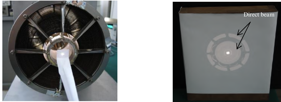
Figure 15. Focal images without the Fresnel Lens. Left: single reflection from the first cone. Right: single reflection from the second cone.
