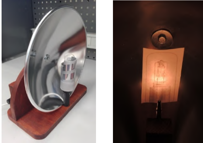
Figure 5. Left: The aluminum tube is blocking the lower part of the source. Right: the higher part of the source is imaged in the lower part of the screen.
