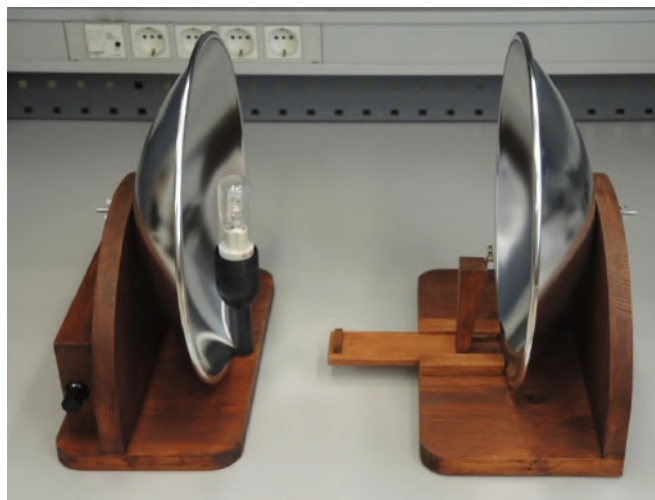
Figure 1. The two parabolas positioned face-to-face to illustrate the normal incident reflection.
