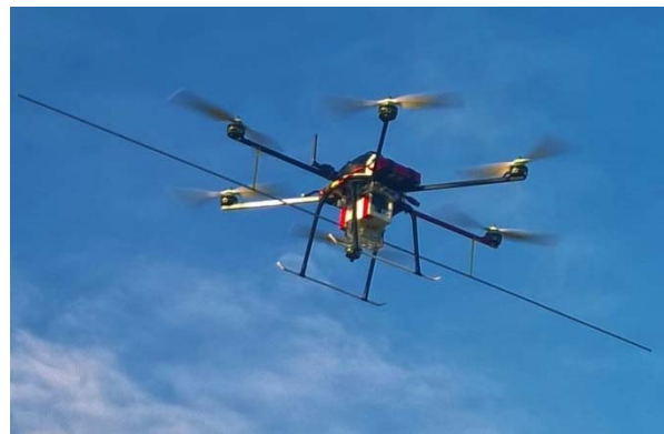
Figure 1: The micro-UAV equipped with RF transmitter, dipole antenna and GNSS system.
