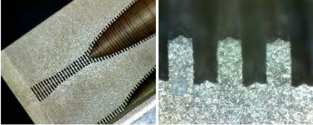
Figure 7. Left. A section of the first feed-horn prototype. Right. Detail of the cusps on teeth and grooves resulting from non uniform chemical erosion.
