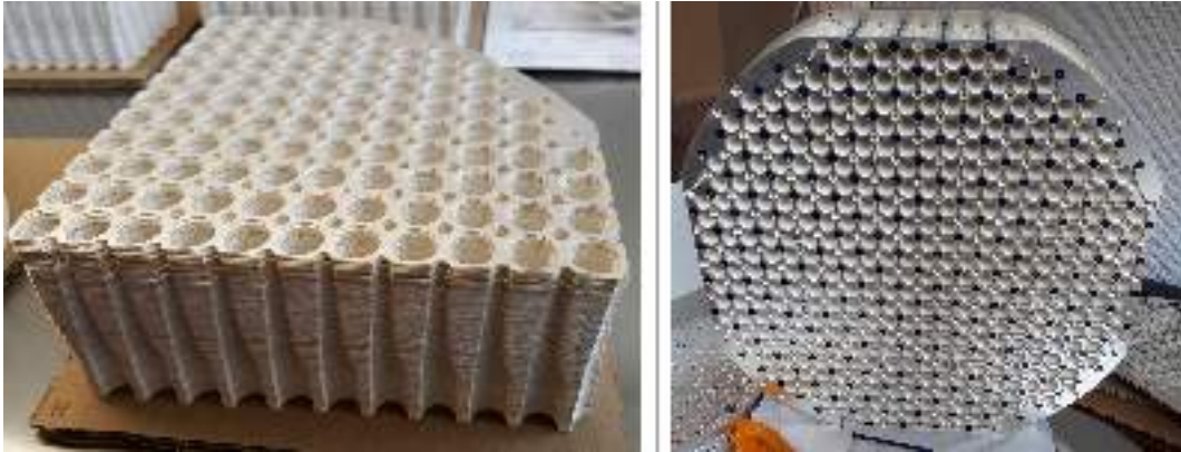
Figure 19. The back-to-back feed-horn system of the QUBIC FI. Left: Stacked platelets of a quarter array. Right: one of the two 400 horn arrays.
