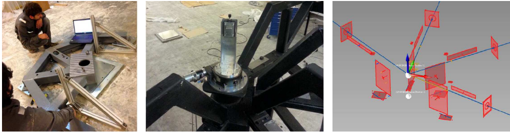
Fig. 1. From left to right: (a) balancer and plates during alignment; (b) detail of the Front End structure with the mode selector and the pentaprism; (c) Front End structure interfaces.
