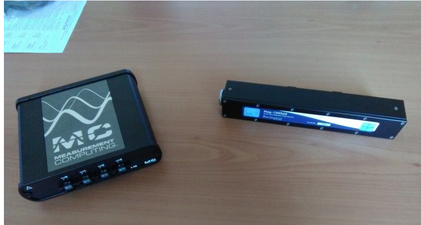
Figure 9. The 3-axis Flux-Gate Magnetometer (right) procured from Bartington Instruments LTD (model MAG-13MS60), and the 4-channels ADC controller (left) procured from Measurement Computing (model USB-2404) for the measurement of local geomagnetic disturbances.
