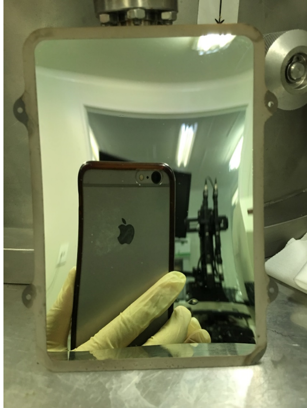
Figure 7. Full-scale LAD filter prototype, mounted in its support Ni frame. From Ref. 5
