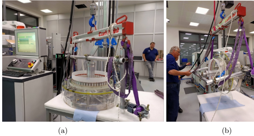
Figure 5: The handling tool used to install the shell on the lathe. A central tube is connected to the spider and is used as connection to the system, so that no deformation is expected on the shell support system. a) Initial configuration, with shell optical axis in vertical direction. (b) Ready for the transfer, with the shell optical axis in horizontal direction.
