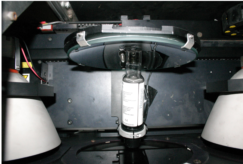
Figure 10. New ThAr lamp and special reflector installed in the calibration unit between other two conventional lamp reflectors.
