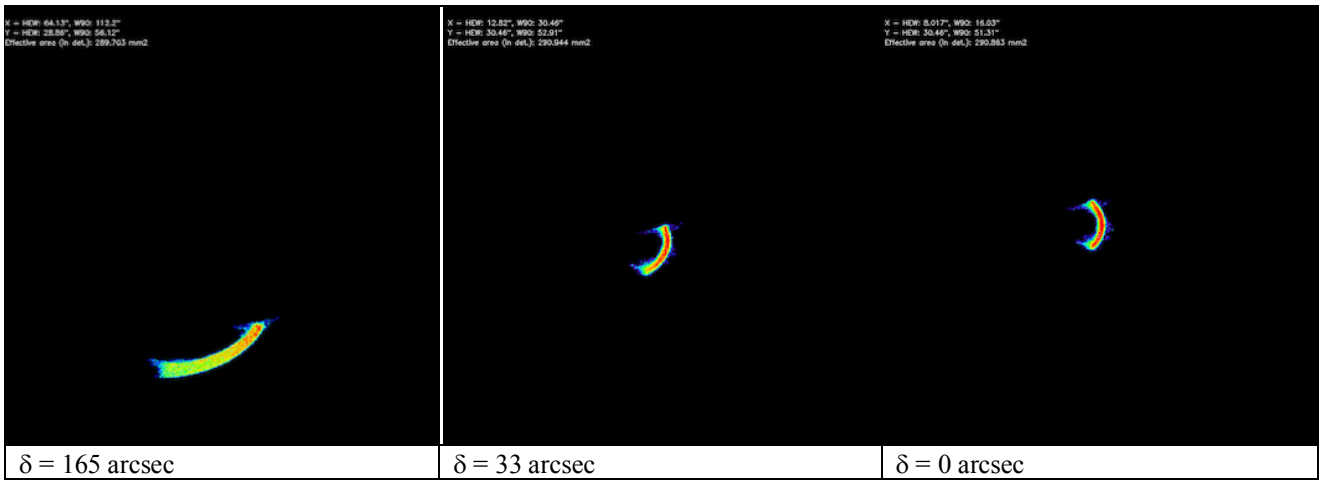
Figure 11: simulated alignment of the yaw angle \delta , if the pitch angle and the focal distance are NOT aligned off-axis, with the diverging beam at 1.49 keV. This time, a pitch misalignment \theta = +83 arcsec was added.
