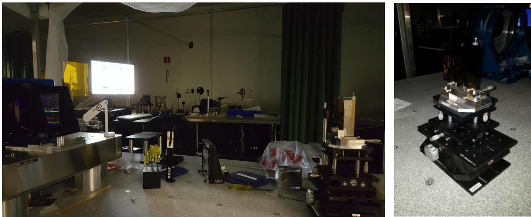
Figure 2: (A) The measurement set-up for the glass plate figure errors available at SAO. The interferometer beam is adapted to the cylindrical geometry with a CGH system. (B) The glass plate is supported on two points on the bottom and one on the top back.
