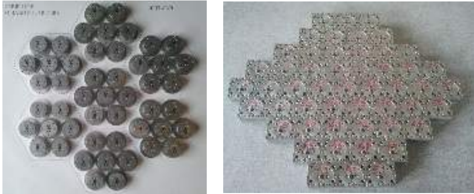
Figure 8. Left: the 49 Strip Q-band polarizers arranged according the 7-module feedhorn footprint. Right: the 49 Strip Q-band platelet OMTs.
