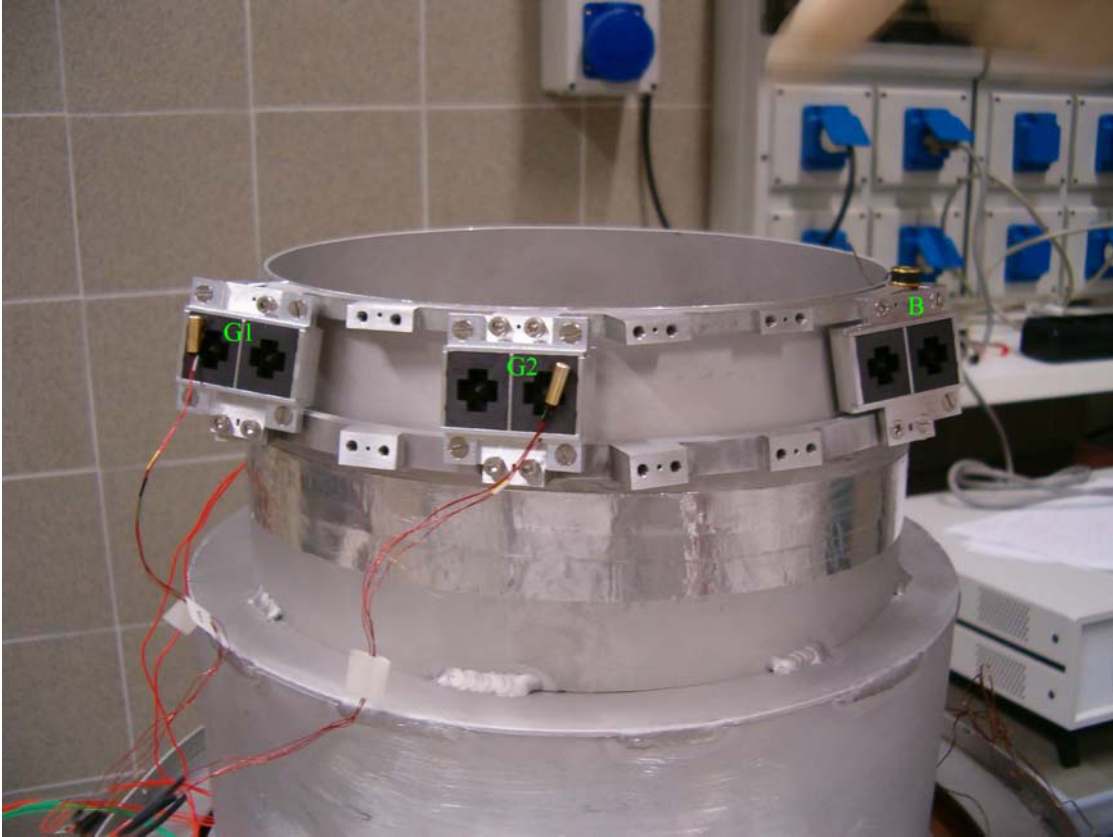
Fig. 47 Experimental setup for 70 GHz RL QM thermal tests. Sensor locations are shown.
