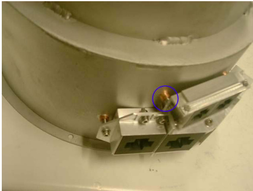
Fig. 12 The sample is mounted on the shield by means of two stainless steel screws and washers fitted to the cylindrical wall by means of copper adaptors (blue circle).
