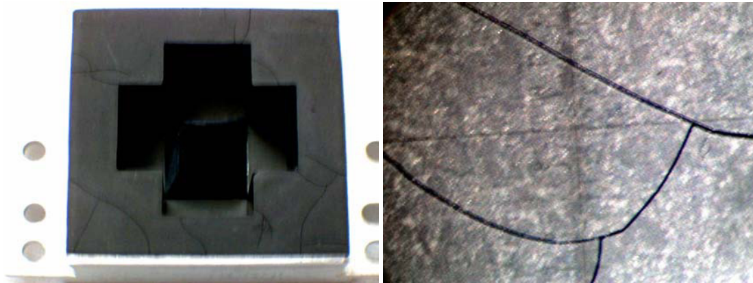
Fig. 45 Cracks on the lateral 30 GHz target (left) and detailed microscope view (right)
