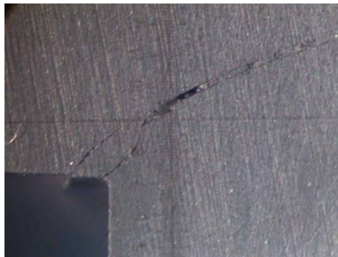
Fig. 46 Microscope image of the 44 GHz crack
