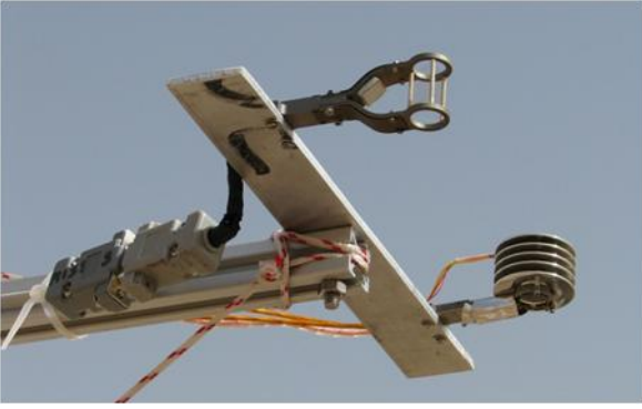
Figure 2. MarsTEM temperature subsystem. On the far left the MISSUS temperature sensor without the shield; on the right side the MarsTEM sensor protected the aluminum shield. On top, fixed to the shield, the PT100 B sensor and in the shadow of the shield the PT100 A, directly exposed to air.
