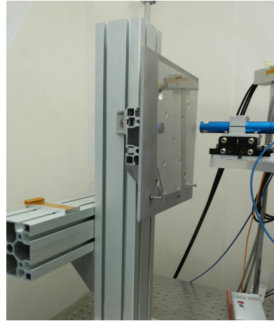
Figure 2: (A) Measurement set-up for glass thickness variation. 100 mm diameter BK7 reference mold used to close the cavity. (B) 3d measurement of plates figure errors.
