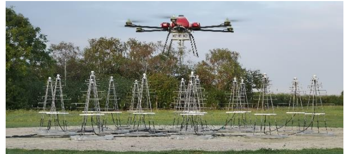
Fig. 1. UAV flying over the preAAVS1 array (SKALA-2 antennas), deployed at the Mullard Radio Astronomy Observatory, Lords Bridge, Cambridge
