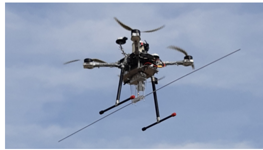
Fig. 3. The UAV-mounted dipole hovering during the measurement.
