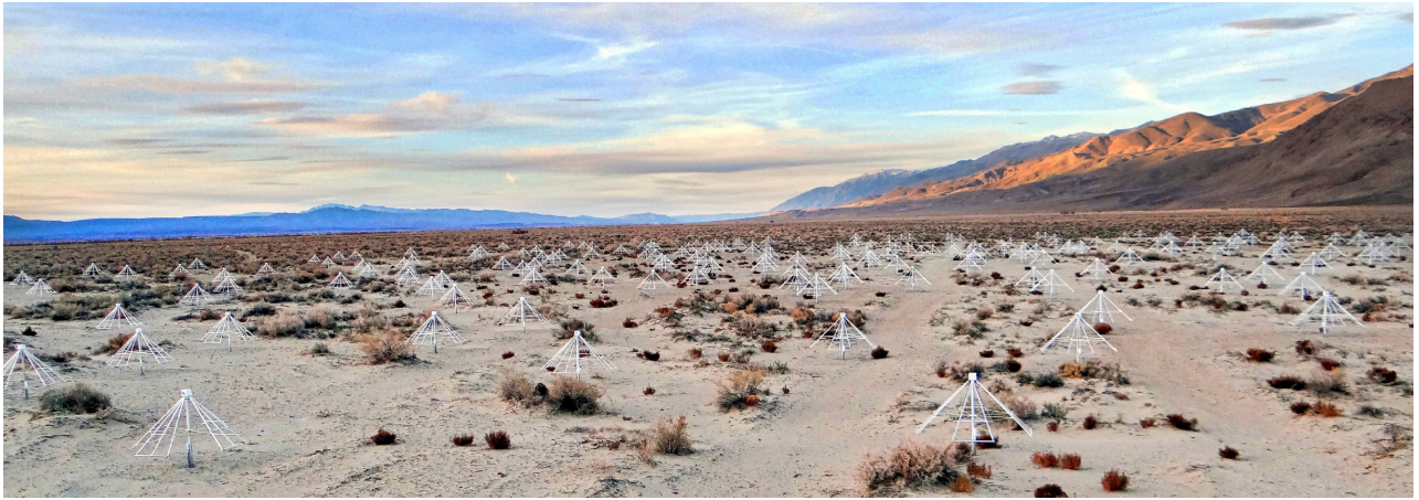
Figure 3. The core area of the Owens Valley LWA, looking north from the electronics shelter located at the edge. The dual-polarization dipoles are aligned north–south and east–west.
