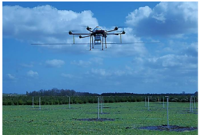
Fig. 3. The UAV-mounted field source flying on the LBA inverted-V dipoles
