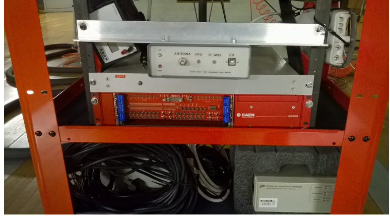
Figure 2. Left : Aqueye+ mounted at the 1.8 m Copernicus telescope in Asiago. The MPD SPAD detectors are visible at the bottom. Top : The heart of the Aqueye+ timing system, leaning on an independent chart: TDC CAEN electronics (red rack at the center), Trimble GPS unit (small gray case on the top), and Stanford Research Systems Rubidium clock (bottom right). The 10 MHz signal from the Rubidium clock is sent to a signal multiplier (big gray case leaning on the top of the CAEN rack), that delivers a 40 MHz reference signal to the acquisition electronics.
