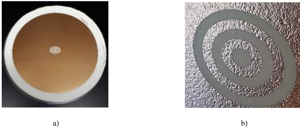
Figure 10. a) The embedded Toraldo pupil prototype operating in the W-band; b) Close-up view of the embedded TP sample.
