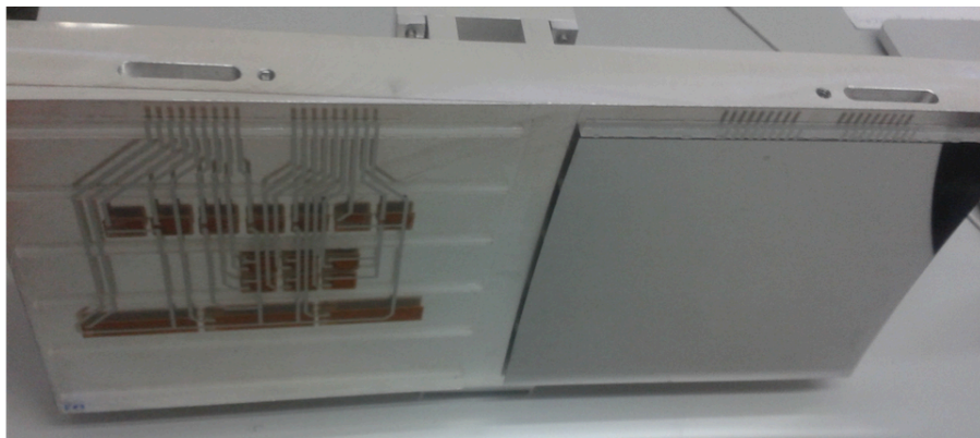
Fig. 4: the complete XMP. The two segments are in Wolter-I configuration but have been tested separately under X-rays. The parabola (on the right) was coated with a thin layer of titanium to enable profile measurements with the LTP and so understand if the deformations induced by the active elements are sufficient to perform the local shape correction. The hyperbola (on the left) has been left uncoated to avoid some possible deformation caused by the stressed coating.
