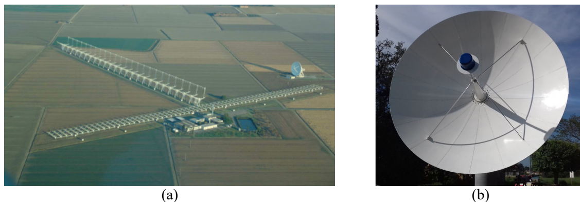
Figure 1: BIRALES sensor. (a): Medicina radio astronomical station located in Medicina (Italy); (b): Radio Frequency Transmitter (RFT) located at the Italian Joint Test Range of Salto di Quirra in Sardinia (Italy).
