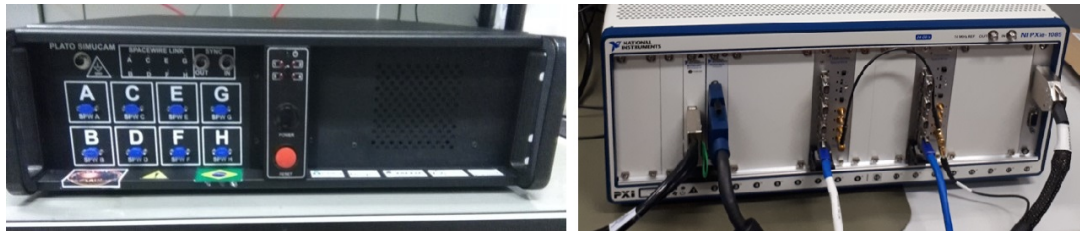
Figure 4. On the left the DPS simulator (SIMUCAM) on the right the spacecraft simulator (SIS)
