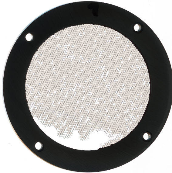
Fig. 52 – Scanner image in transmission mode of the sample filter M1 at the end of the S5/R5 level vibration tests.
