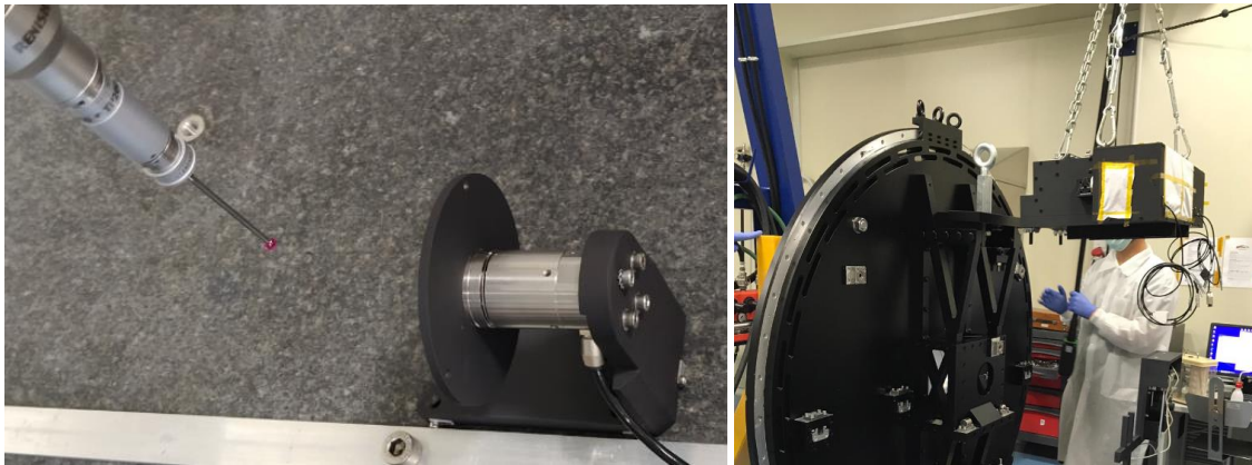
Figure 10. Left: NIR tip-tilt mirror during the CMM verification process. Right: installation test on the interface flange.
