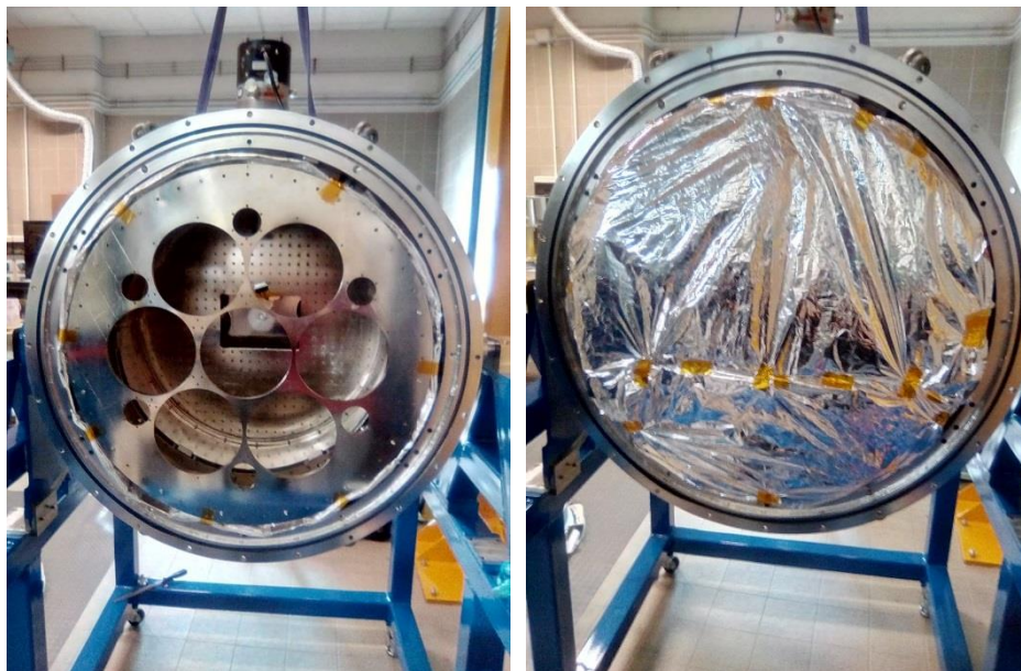
Figure 7 The filter apertures on the top of the 80K cover (left) have been closed by thermal MLI blankets in order to shield radiative loads on the colder part of the cryostat.
