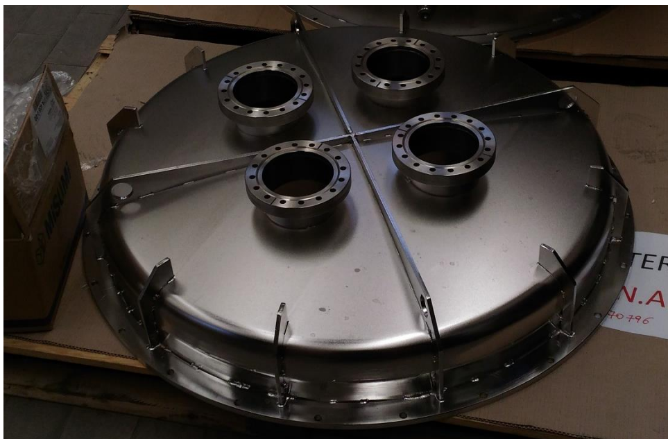
Figure 4 Top panel: the top cover of the cryostat with the window aperture. Bottom panel: The bottom cover of the cryostat with the apertures for the vacuum bench connection flanges and spare connector flanges.
