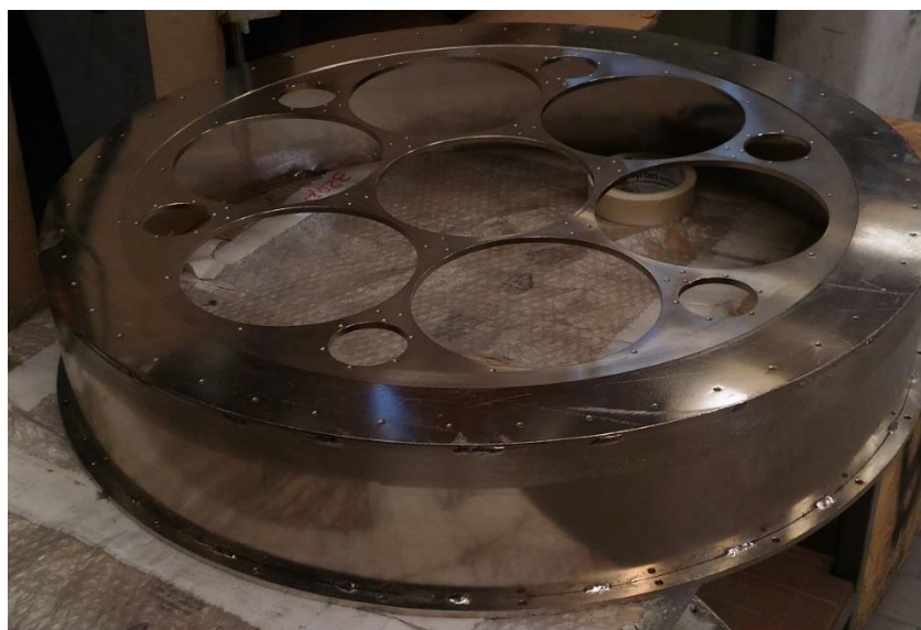
Figure 3 The top part of the 80K shield with the apertures dedicated to host the thermal filters.
