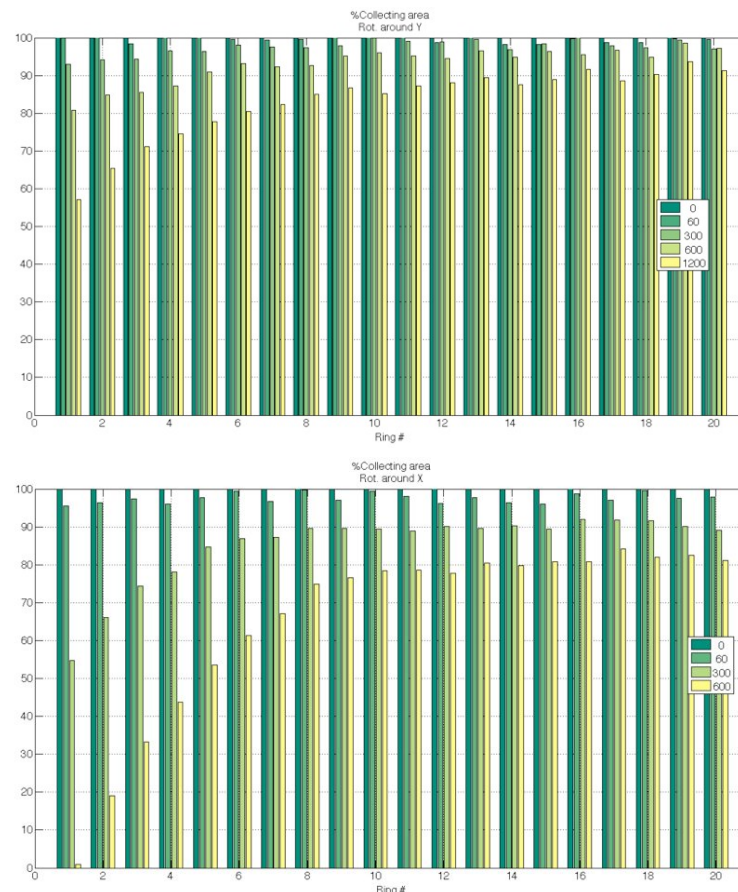
Figure 10. Percent of residual collecting area with respect to the on-axis configuration for different rotation amplitudes (0 , 60, 300, 600, and 1200 arcsec). Top: rotation around y -axis. Bottom: rotation around x -axis.
