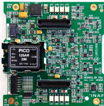
Figure 10 Left: Demonstration model of the HERMES-TP/SP Power Supply Unit (PSU). Right: schematic block diagram of the PSU
