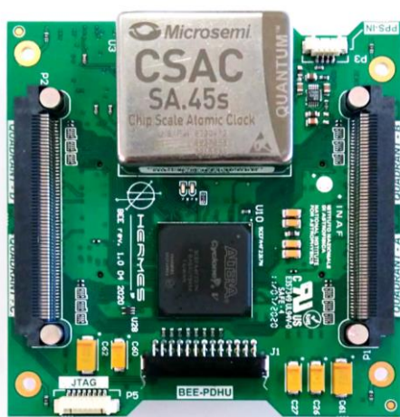
Figure 9 Left: Demonstration model of the HERMES-TP/SP back-end electronics PCB. Right: schematic block diagram of the BEE
