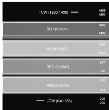
Figure 8 The 6 defined windows for the FPA (4 filters and the 2 in black masked area).
