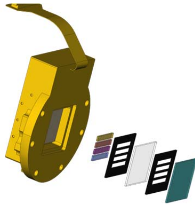
Figure 5 CaSSIS filter layers sequence as it is the flight the detector from the telescope side (AR coating, black mask, fused silica layer, Black Mask, 4 passband coatings)
