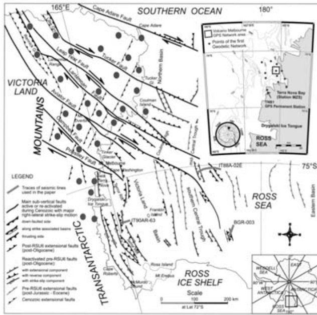
Fig. 1. Suitable spots (dark dot) chosen for GPS measurements on the Cenozoic Tectonic Map that represent the Ross Sea Region. From Salvini et al. (1997) with modifications. The inset in the upper right corner depicts a location map of the points belonging to the first geodetic network (dark dots) and its densification (within the dark frame) around the Mount Melbourne volcanic edifice. TNB1 represents the location of the GPS permanent station.
